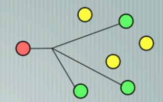
**Multicasting** allows sending a single image simultaneously to many machines without putting greater stress on the network than by sending an image to a single machine.
